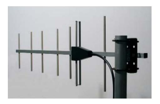
Frequency range 390 - 475 Mhz 50 ohm Impedance **VSWR** < 1,6 Gain 8,5 dBd > 20dB Front to Back ratio VERT./HOR. Polarization Maximum power 100 W Connector 1.5 m RG-213 + N Width 35 cm 105 cm Length Mass of antenna 2,5 kg
