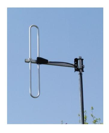
118 - 136 MHz Frequency range 50 ohm Impedance **VSWR** < 1.5 Gain 0 - 2 dBd VERT. Polarization 500 W Maximum power Connector Ν 1100 mm Height Lenght 700 mm 2.5 kg Weight 160 km/h Wind velocity
